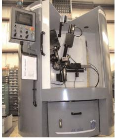
A FITCAL checklist, shown here in plastic sleeve on this AL805, is a tried and true, easy way to remember six basic maintenance operations every grinding shop should do to prevent breakdowns and interruptions in service.
